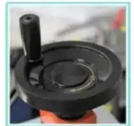
Marking the rotation direction sticker on hand wheel, which is convenient for adjustment.
