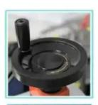
Marking the rotation direction sticker on hand wheel, which is convenient for adjustment.
