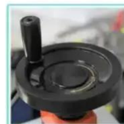
Marking the rotation direction sticker on hand wheel, which is convenient for adjustment.
