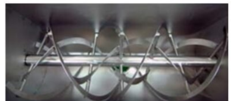
RM-100 DOUBLE RIBBON AGITATORS INNER CONSTRUCTION
