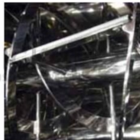
► INNER MIXING BLADE WITH SCRAPER
