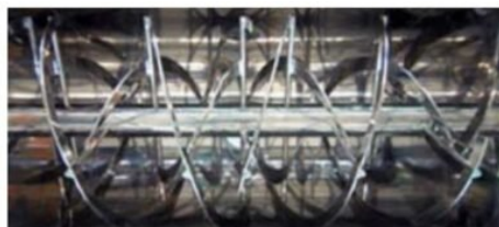
RM-500 DOUBLE RIBBON AGITATORS INNER CONSTRUCTION
